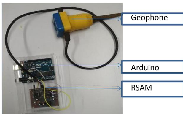
Figure 3. Electronic module of the RSAM system
