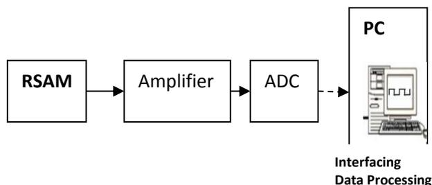
**Figure 1.** Block computerized RSAM system diagram
